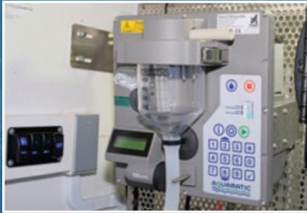
**Aquamatic Composite and Discreet Samplers** – These wall mountable models offer simple operation, combined with rugged construction and excellent reliability. The samplers have a main power connection and an integral 12 VCD battery. The units come with 30 feet of sampling hose, battery charger and weighted strainer.
