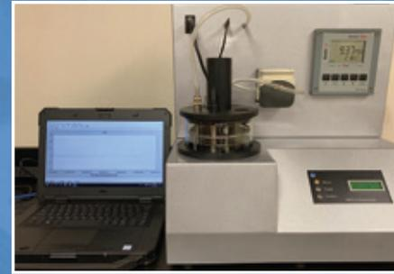
**Surgis Field Respirometer** - Surgis BM respirometers are compact, simple, and user friendly, with very low maintenance. Each unit is equipped with powerful software that measures key parameters on the actual wastewater treatment process, enabling operators to better evaluate factors such as nutrients, biomass, pH, temperature, retention time, and dissolved oxygen to see the overall impact on the plant's microbiological growth.
