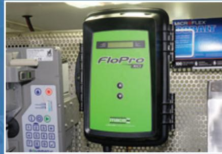
**Flow Monitoring and Data Collection** – The FloPro XCI from Mace provides for measurement of velocity, flow, depth, and use of a multi-parameter water quality sonde. The unit is a smart package monitoring solution that provides remote data access with alerts and alarms. It is telemetry-ready for effective, low-cost control and rapid response.
